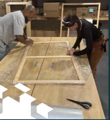
\* Each insert features a pine frame that is custom-built using the exact measurements of each window. This frame is wrapped tightly on both sides with poly olefin film, sealed, and finished with a foam gasket.
